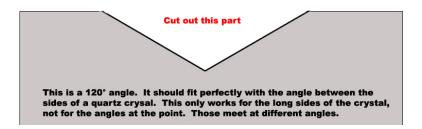
Carefully cut out the gray area, being especially careful to stay with the lines as you cut out the notch on the top. That will give you an angle of exactly 120°, which will match the angles between the six sides of a hexagonal quartz crystal.
